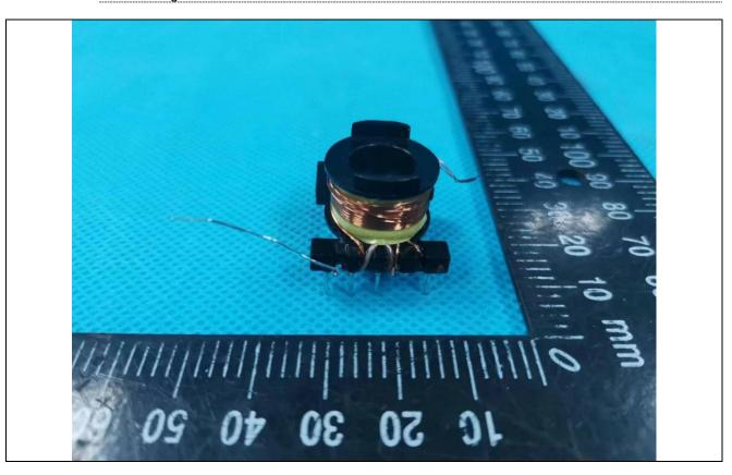
Details of: Secondary view for N3 winding of T1
